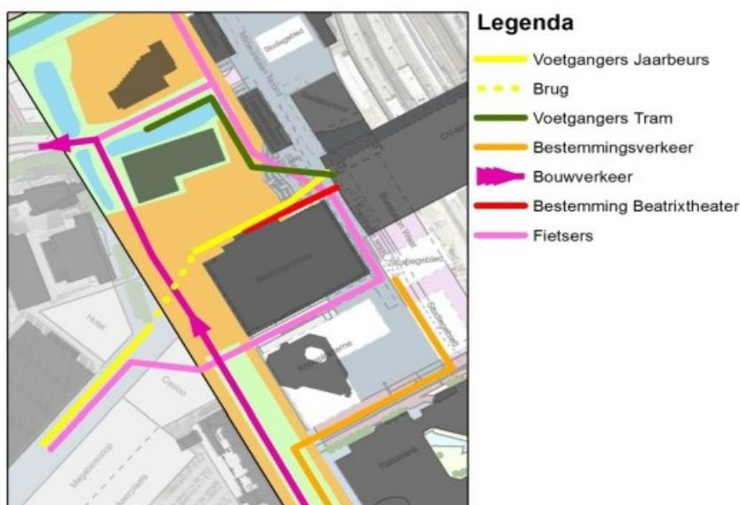
**Figure 4** Alternative routing for different traffic flows during construction at the Jaarbeursplein
